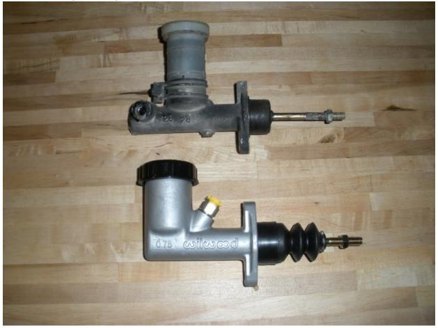
Step 1: Disassemble both master cylinders Remove the boots from both master cylinders.
